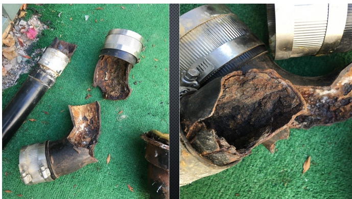
Cast iron corroded pipe
